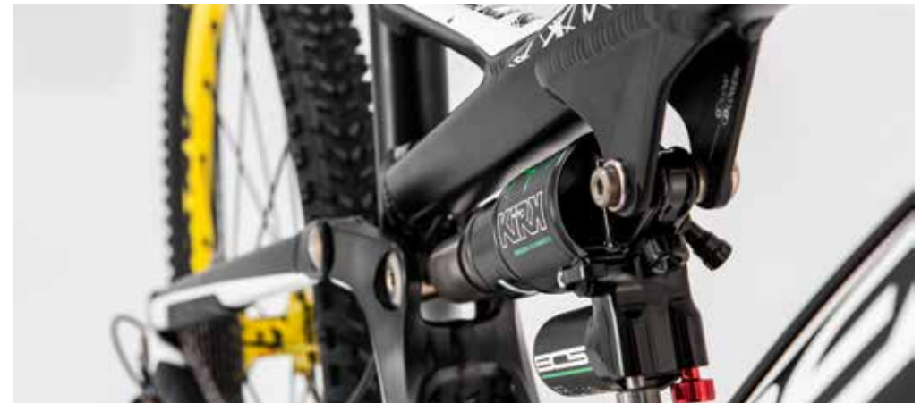
PRESSURE AND REBOUND CLICKS: The values provided in the chart are just a starting point, in order to achieve maximum performance the shock setup should be suited to the rider and terrain. COMPRESSION ADJUSTMENT FOR KIRK SHOCK: 12 clicks counted from completely open is the recommended starting point both for low speed and high speed compression damping.
