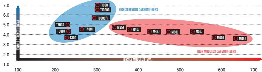
This sample diagram of products from Toray Industrial is a good illustration of the types of choices available to our carbon engineers. Orbea uses various grades of carbon from multiple manufacturers to tune the ride of each frame. We notice how extremely high-mod (stiff) fibers become less strong over time, so in order to take advantage of their properties it is necessary to blend them with more flexible, high-strength fibers.
