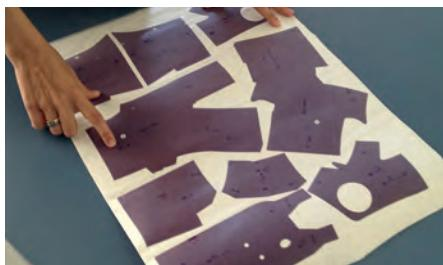
To make the lightest frames, prepreg is laser-cut into shapes that use only the optimum amount of material
