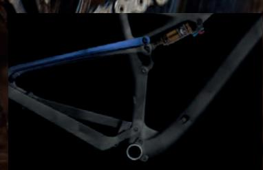
Total deflection of the swingarm requires less than 5kg of force on the saddle compared to 250kg required to fully compress the shock.
