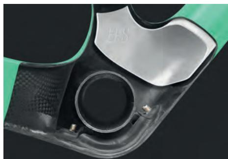
The smooth interior surface of an EPS-molded frame
