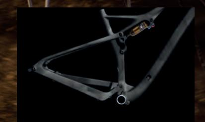
The swingarm flexes upward as the linkage moves
