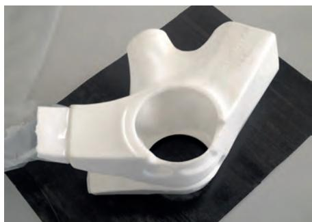
A polyurethane form helps improve compaction and reduce wrinkles in frames molded with bladders
