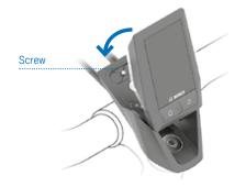
To remove the Kiox display from OC Components holder, unscrew first the bolt on the back of the holder with a 2.5mm Allen key.
