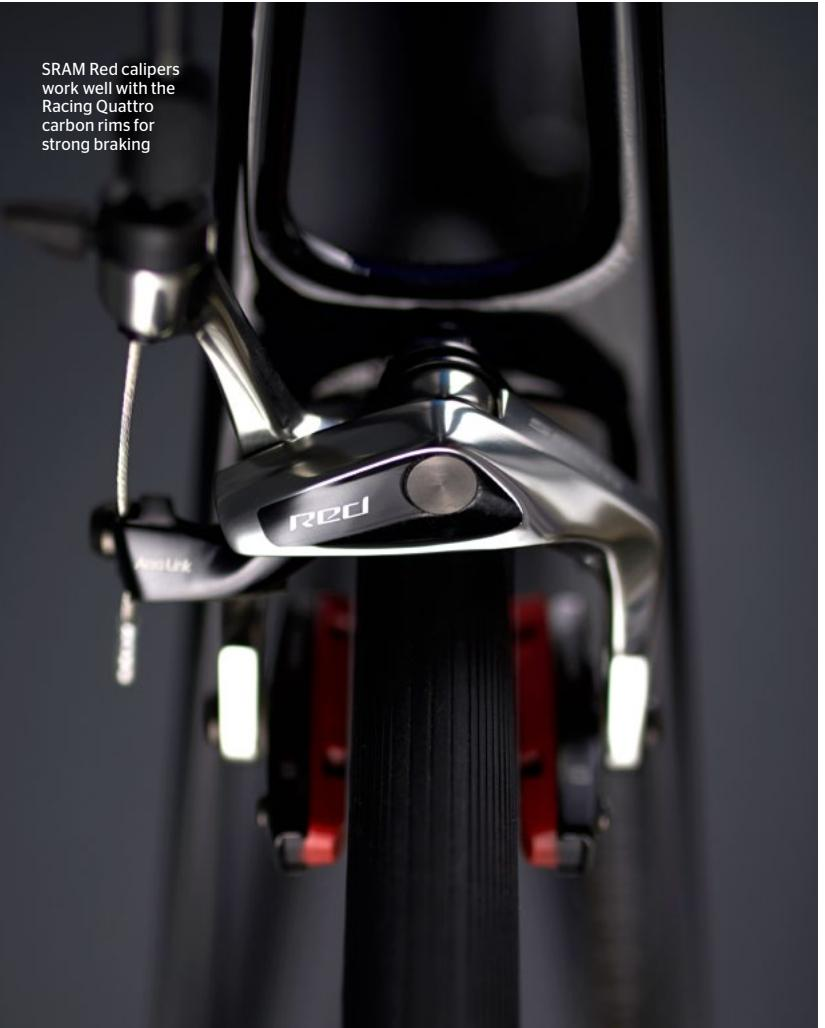
SRAM Red calipers work well with the Racing Quattro carbon rims for strong braking
