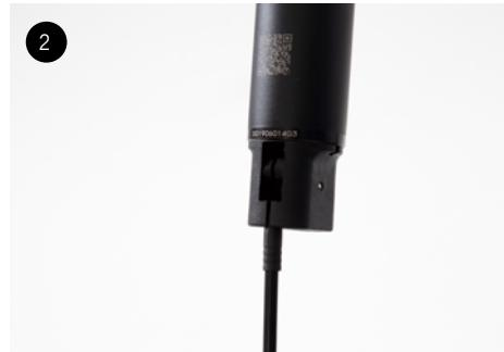
Install a 4mm plastic ferrule on the outer cable end coming out of the seatpost. Insert this end of the outer cable into the seatpost actuator's housing.
