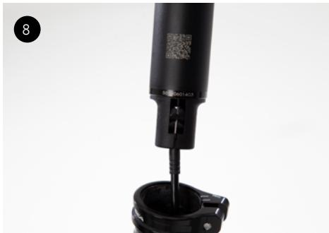
Install the gear cable's head into its housing on the seatpost actuator and insert the outer cable into its housing on the seatpost base.
