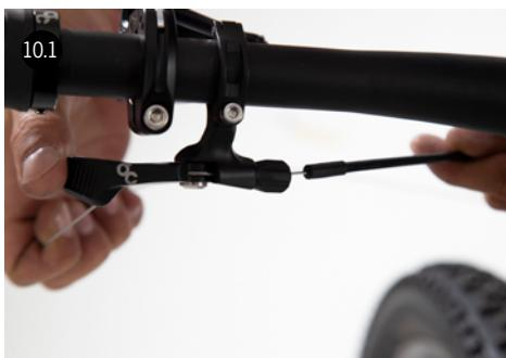
Guide the cable through the remote's barrel adjuster and through the hole on the lever. Lightly pull from the cable to remove any slack and tighten the lever setscrew (1,2Nm). Cut the cable and install a metal cable end.
