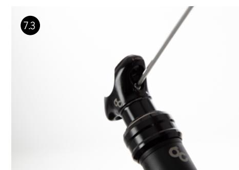
Completely insert the hydraulic cartridge into the seatpost assembly so the notch on the top of the cartridge is aligned with the setscrew on the back of the seatpost head.
