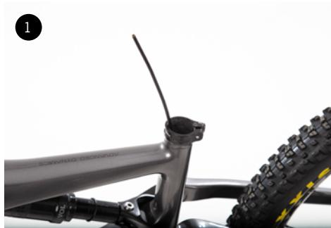
Install the outer cable into the frame following the frame's specific routing. Introduce it into the port on the front of the bike and guide it until it comes out of the seat tube. 20-25cm should protrude out of the seat post.
