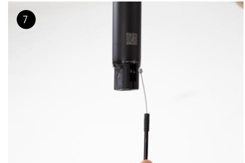
Insert a gear cable into the outer cable from the seatpost end.
