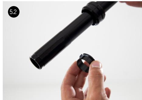
Remove the lower and upper bushing from the upper seatpost assembly.
