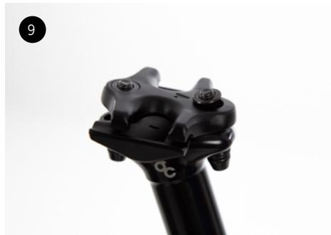
Insert the seatpost into the seat tube while carefully pulling from the outer cable from the front of the bike until the seatpost is at the desired height. The arrow on the saddle clamp should point to the front of the bike.
