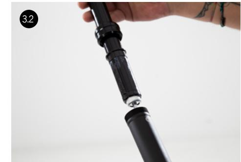
With your bare hands, unscrew the seal collar ring and remove the outer tube from the upper tube assembly.
