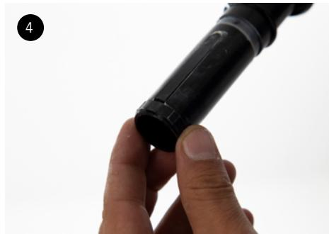
Install the lower bushing, making sure it is seated into the notches on the base of the upper tube.
