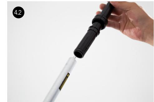
With a 3mm Allen wrench, unscrew the setscrew at the back of the seatpost head. Remove the hydraulic cartridge from the inside of the upper tube assembly. Remove the rubber bottom out bumpers from the cartridge shaft. Clean the cartridge with a soft cloth if you are going to re-use it.
