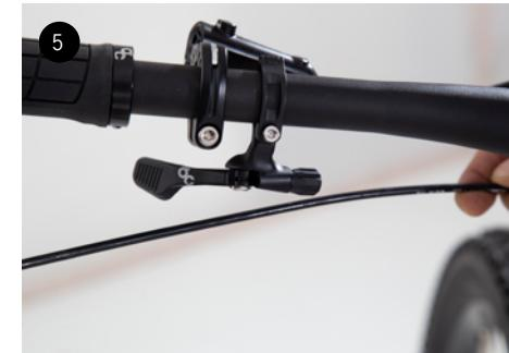
Take the outer cable end at the front of the bike to the remote lever to determine the lenght needed. Turn the handlebar both ways to ensure they turn free all the way and the outer cable does not interfere with other cables or components.
