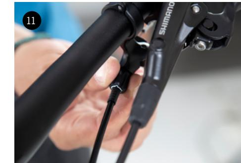
Adjust the cable tension with the barrel adjuster until there is no play on the lever. New cables can develop slack until they completely settle, remove any slack with the barrel adjuster after the first rides.
