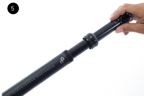
Insert the upper tube assembly into the lower tube. Ensure the guides slide into the notches on the lower tube.
