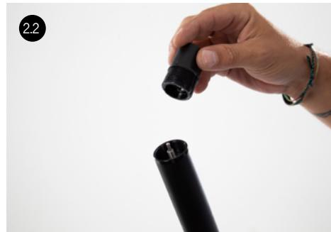
Hold the seatpost with your hand or soft rubber jaws and use a 10mm Allen wrench to unscrew the actuator from the base of the seatpost.
