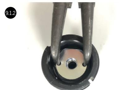
**⚠** Before installing the actuator assembly onto the shaft, and to avoid seatpost malfunction in case the locknut is loose into the actuator housing, remove the locknut from the actuator housing and tighten it onto the shaft using the tool provided in kit F or with the new cartridge. Then install the actuator housing onto the shaft.
