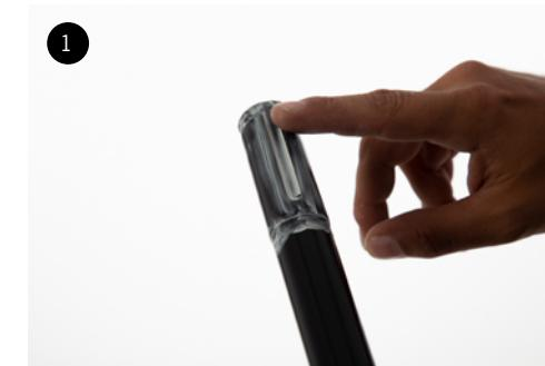
Apply a thin layer of grease on the guides housings and the areas where the bushings will be installed.
