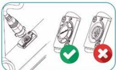
Do not insert metal objects in the charging port or in any of the component connectors. This could damage the connectors or even short-circuit the system.
